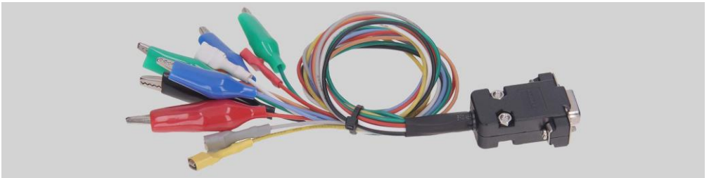
Figure 4 – Diagnostic cable for voltage regulators MS-33502
